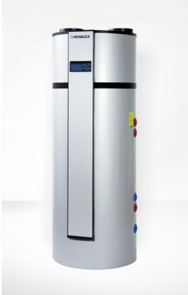
HEWALEX PCWU 200K / 300K / 300SK-2.3kW heaters with heat pumps are intended for heating domestic water in households using air heat pump integrated with the heater. As standard, PCWU heat pumps are also equipped with electric heaters.
